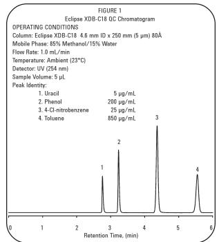
The uniform, spherical Eclipse XDB-C18 particles are based on Zorbax Rx-SIL silica support that has a nominal surface area of  $180~\text{m}^2/\text{g}$  and a controlled pore size of 80Å. Columns are loaded to a stable, uniform bed density using a proprietary, high-pressure slurry-loading technique to give maximum column efficiency.
